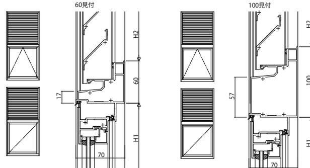
(4 9) F I X窓(内押縁・外押縁)／外開き窓・たてすべり出し窓
